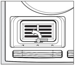
■ Turn the lever on the condenser unit upwards to the vertical position so that the hook on the lever is no longer in the groove at the bottom of the condenser unit housing.
